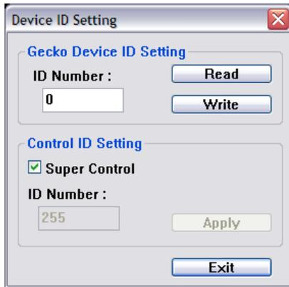
1. Assign an ID for the connected MX-1003B: type a number in the “ID Number” of the device ID setting area and then click “Write”.
